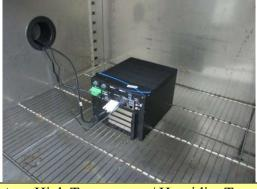
High Temperature/ Humidity Test; Low Temperature Test
